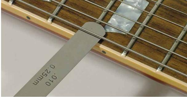
To measure for proper truss rod tightness, an automotive-style thickness gauge and straightedge are needed. As it turns out, a string under tension happens to make a very good straightedge. The process therefore involves holding the string down at the two extreme frets and measuring clearance between the string and fret at the midway point. Since you only have two hands, a capo is provided for the first fret. Fasten the capo on top, rather than behind, the first fret.
